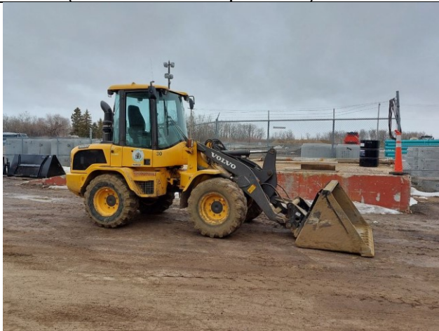
Volvo L35GS Loader Used as a chase loader and for loading sand/salt
