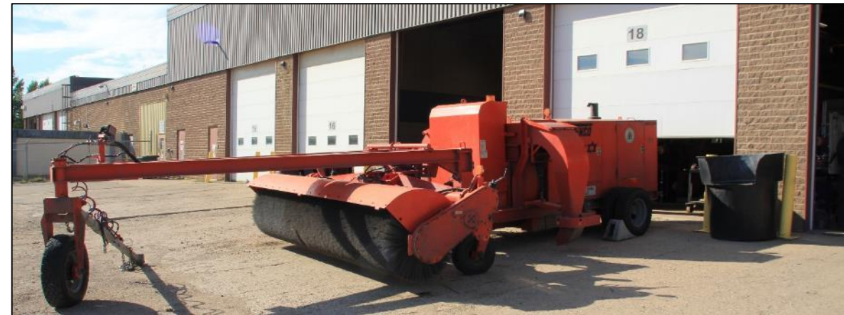
Towed sweeper being maintained by the Fleet Division
