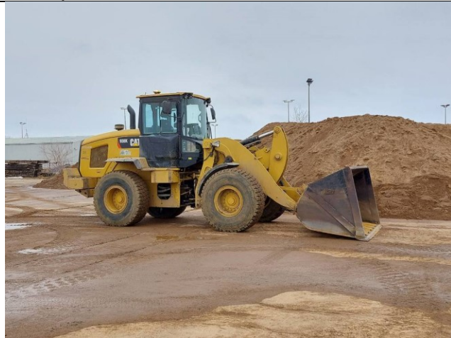
Caterpillar 938K Loader Used as a chase loader, cleaning corners and cul-de-sacs
