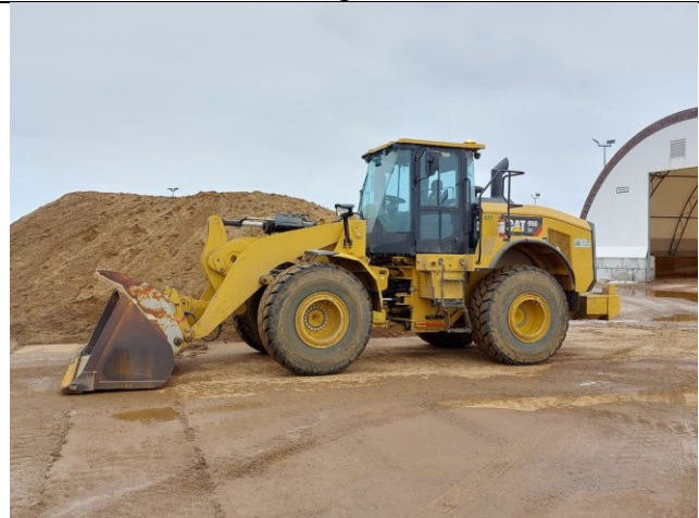
Caterpillar 950 Loader Used as a chase loader, cleaning corners and cul-de-sacs or for the snowblower
