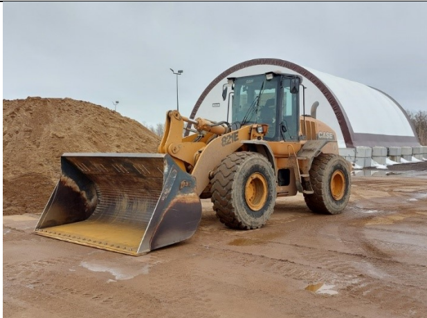
Case 821E Loader Used as a chase loader and for loading salt/sand
